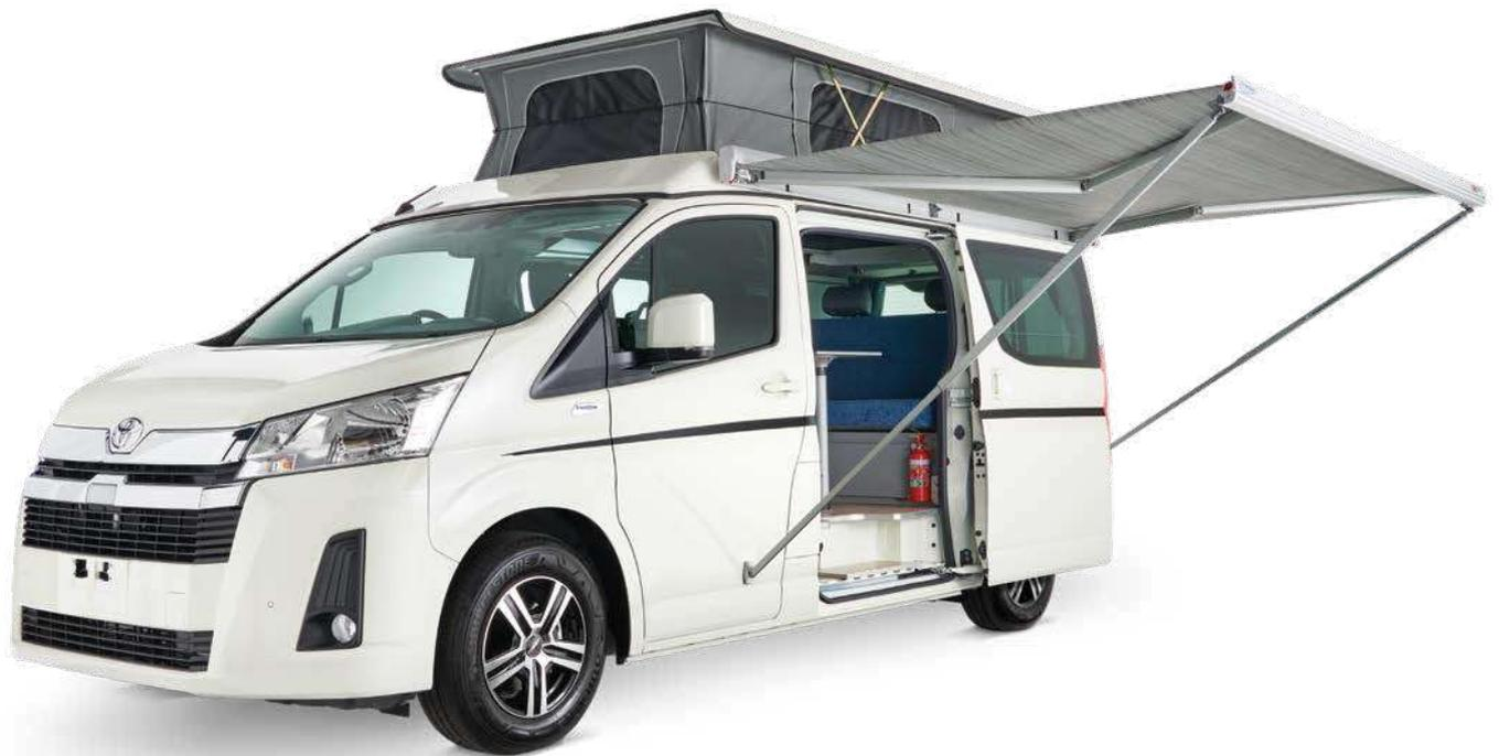
A significant development is the bonneted body style that places the engine up front, providing increased front end collision protection. Being seated behind the engine bay, allows for comfortable bucket seats for increased comfort, plus a walk-through cabin for increased functionality. With further improvements to safety, the HiAce now includes seven airbags and obtains a 5-star ANCAP rating.
